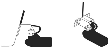
Route cable through bracket and mount transducer, side view (left) and seen from above (right).
